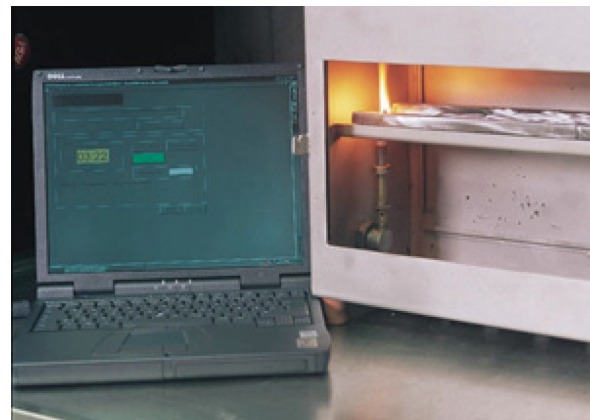
Figure 4 - FMVSS 302 – Horizontal burning rate determination. Credits ©Currenta
