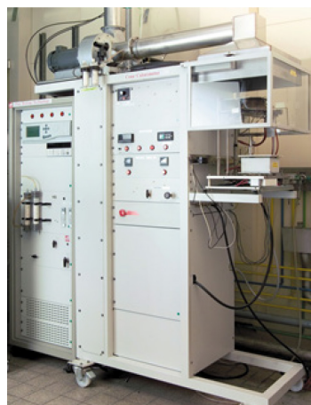
Figure 6 - ISO 5660-1 – Cone Calorimeter. Credits ©Currenta
