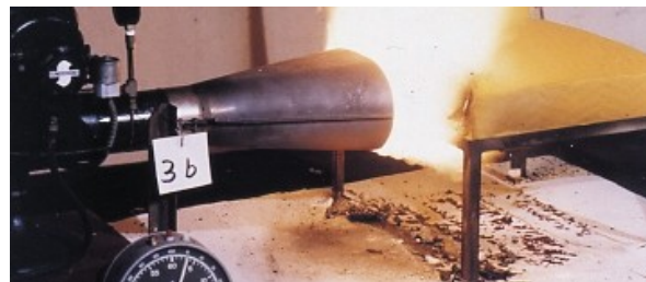
Figure 11 - Oil burner for seat cushion flammability test. Credits ©Currenta
